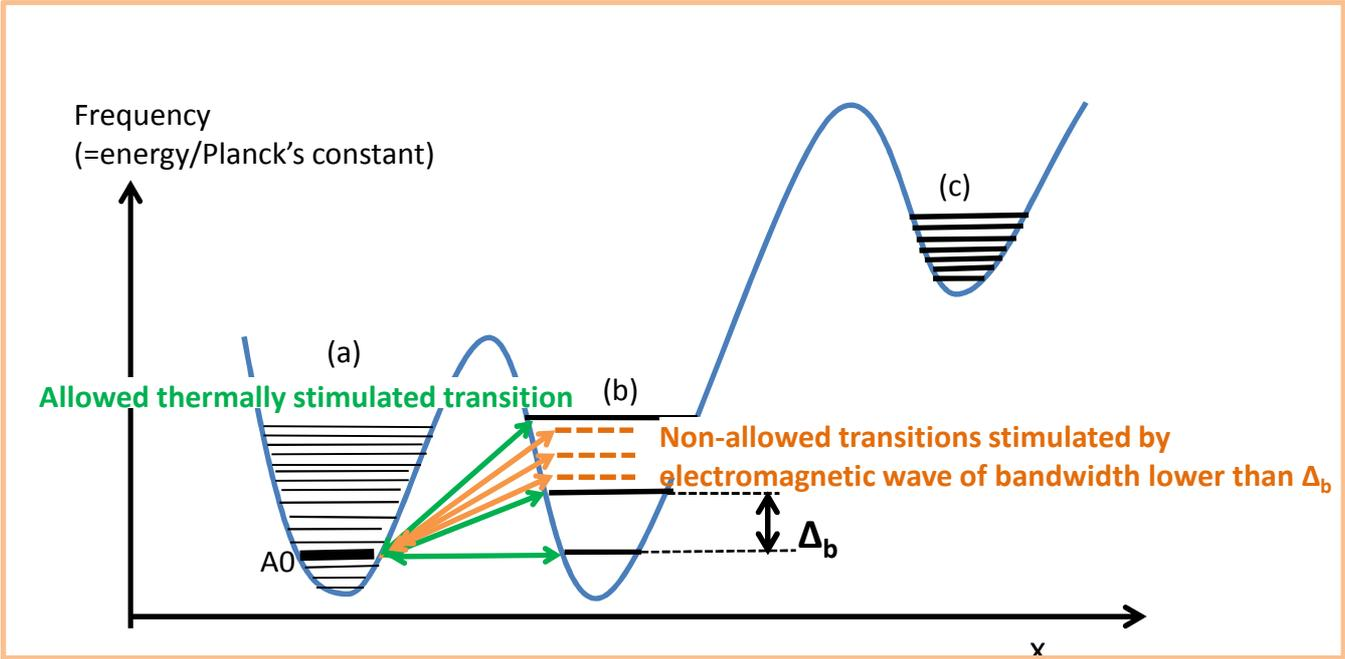
Figure B4: Transitions from quantum state A0 to quantum states in well (b) cannot be stimulated due to insufficient bandwidth; Transitions from quantum state A0 to well (c) are therefore not inhibited. Inhibition of transitions from (a) to (c) is incomplete and strongly limited.
